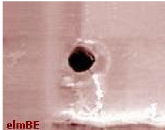
Figure 6 - Photo of an ESD-induced Oxide Breakdown
